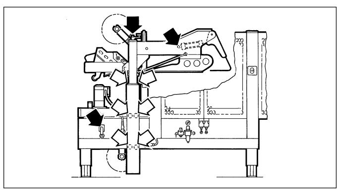
Figure 4-1 – Lubrication Points, Frame
